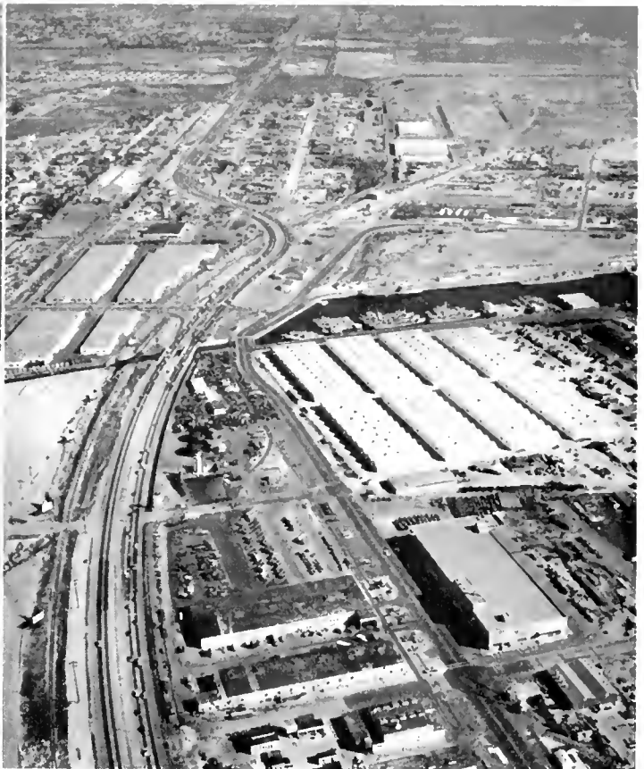
LEFT—Main Street interchange and in distance three-level connection to Palm Avenue. RIGHT—Approaching freeway from North Eighth Street intersection in National City at left center. Curves will be eliminated by adopted freeway routing.
